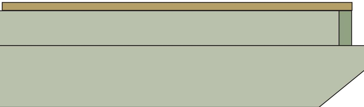
Make sure to have half the joist exposed and that screws do not miss the joist. Give them a little angle.
